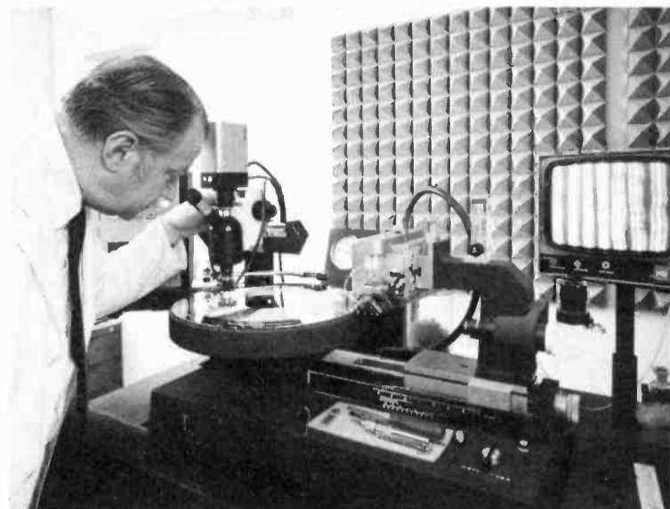
A CUT ABOVE —A technician checks the cut on the copper-plated steel disk used in Teldec's Direct Metal Mastering process. The special stereo cutterhead has been developed by Neumann.
